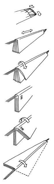
Stretch the parachute completely by holding the lines in each end, the apex and the leading edge.
