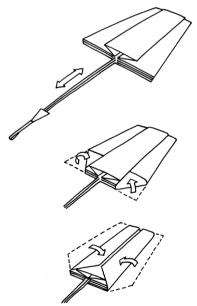
Fold the corners of the canopy, then both sides into the centre and in the last fold open inside gore number 1.
