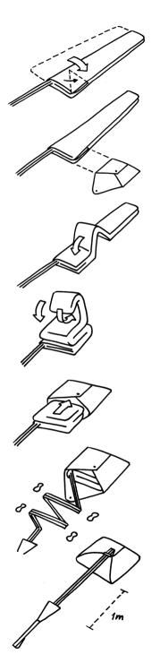
Fold the parachute like an accordion with each fold roughly corresponding to the internal bag size. The last fold should be to the inside. Put the canopy in the internal bag and close it with the hand strap temporarily.
